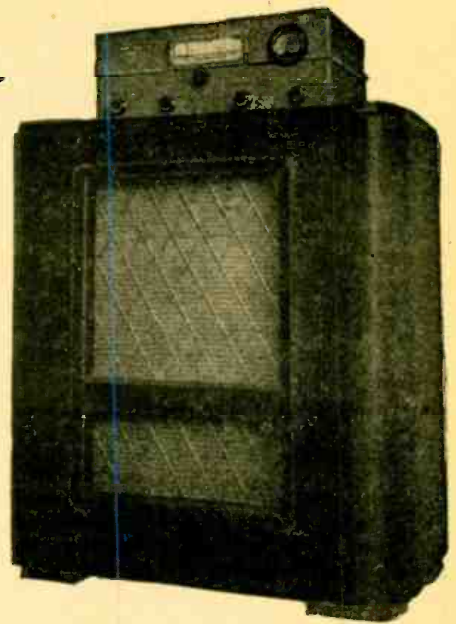
Completed receiver on its bass-reflex cabinet.
