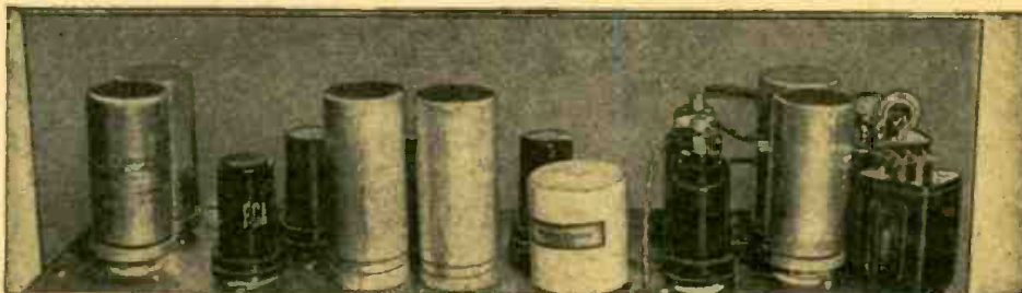
Rear view of preamplifier. There is plenty of decoupling capacity.
